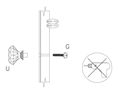
CAUTION: Only hand tighten the handle, overtightening could damage the mirrored drawer fronts.
